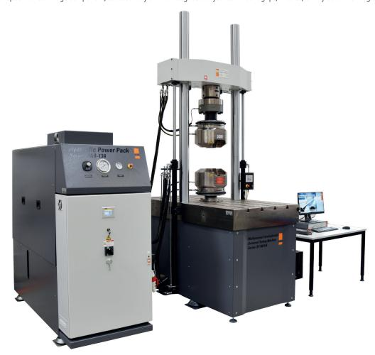
You can also extend your test system to multi-channel; multi-axis testing when adding an additional linear actuator or torque drive. This additional actuator you can mount in the same way as you can mount specimens or subassemblies direct onto the t-slot platen or via reaction bracket, adapter plate or support horizontally or with any inclination onto the T-slot platen.
