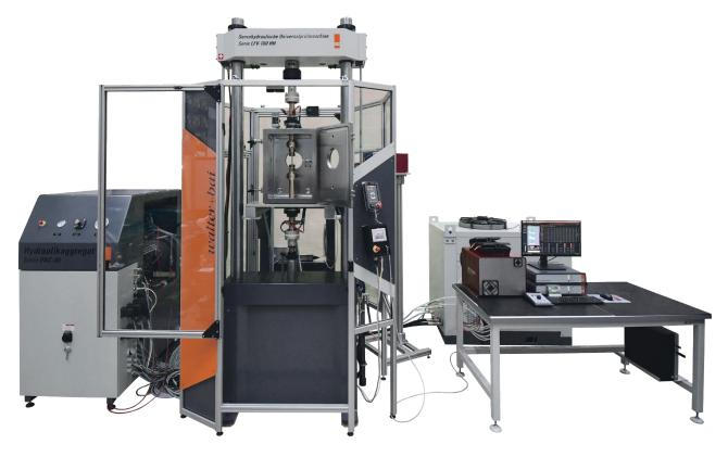
Our LFV test system are easily configured to accommodate electrical resistive high temperature heating system with or without inert gas chamber. These heating systems provide high speed direct specimen heating by passing a low frequency electrical current through a specimen.
