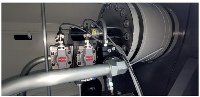
This series of LFV-T test system incorporates the torque-generating high-performance torsional cylinder with hydrostatically supported balanced double-vane rotor design ensur¬ing zero actuator backlash during revers testing and is well suited for high speeds. The system static rated torques are reached at 250 bars.
