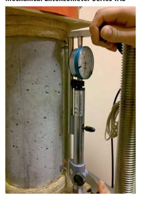
This accurate units are available with standard 20 - 200 mm gauge length and digital gauge with a resolution of 0.001 mm.
