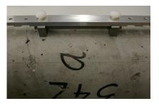
The LVDT and Invar rod is fixed in holders that are glued onto the specimen surface along with the cluing device that enables you to glue the holds with desired gauge length distance.
