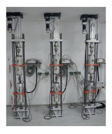
We are also offering Tensile Creep Test Systems for time-dependent tests of concrete <a href="https://www.ncbi.nlm.nih.gov/pmc/articles/PMC6025542/">https://www.ncbi.nlm.nih.gov/pmc/articles/PMC6025542/</a>
