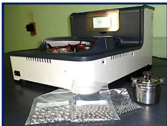
**Fig. 1.** Molino Planetario micro mill PULVERISETTE 7.
